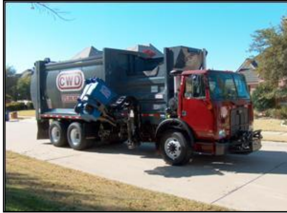
Automated Side Load Truck Emptying 95 Gallon Recycle Cart
